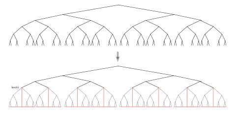
Figure 16.14: For each level-k vertex u, the subtree rooted at u is replaced with the minimal subpath P' of P containing the leaves of that subtree, together with a shortest u-to-P' path. The new subtrees are indicated in red.
