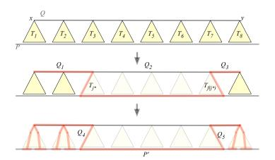
Figure 16.16: The original tree T is shown at the top. It consists of an x-to-y path Q and trees  $T_1, \ldots, T_k$  rooted at vertices of Q. In the first step, the subpath  $Q_2$  and the middle trees are replaced by the paths  $Q_4$  and  $Q_5$  and the subpath P' of P. In the second step, SPAN1 is applied to the non-middle trees.
